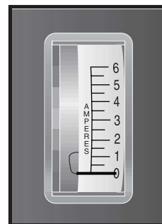
Figure 9. Ammeter Indicates Batteries Are Fully Charged
