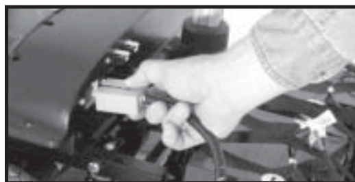
Figure 19. Disconnecting The Front-To-Rear Harness
