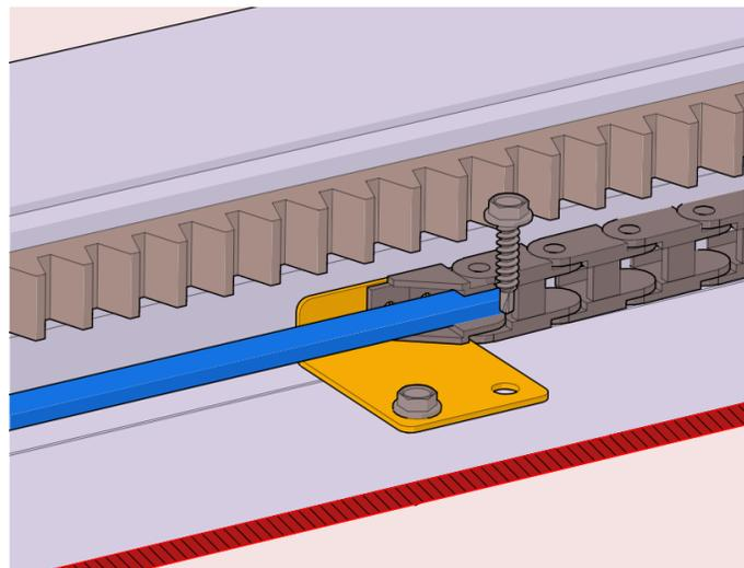
Place the upper limit cam inside the track and secure by tightening the phillips head screw.
