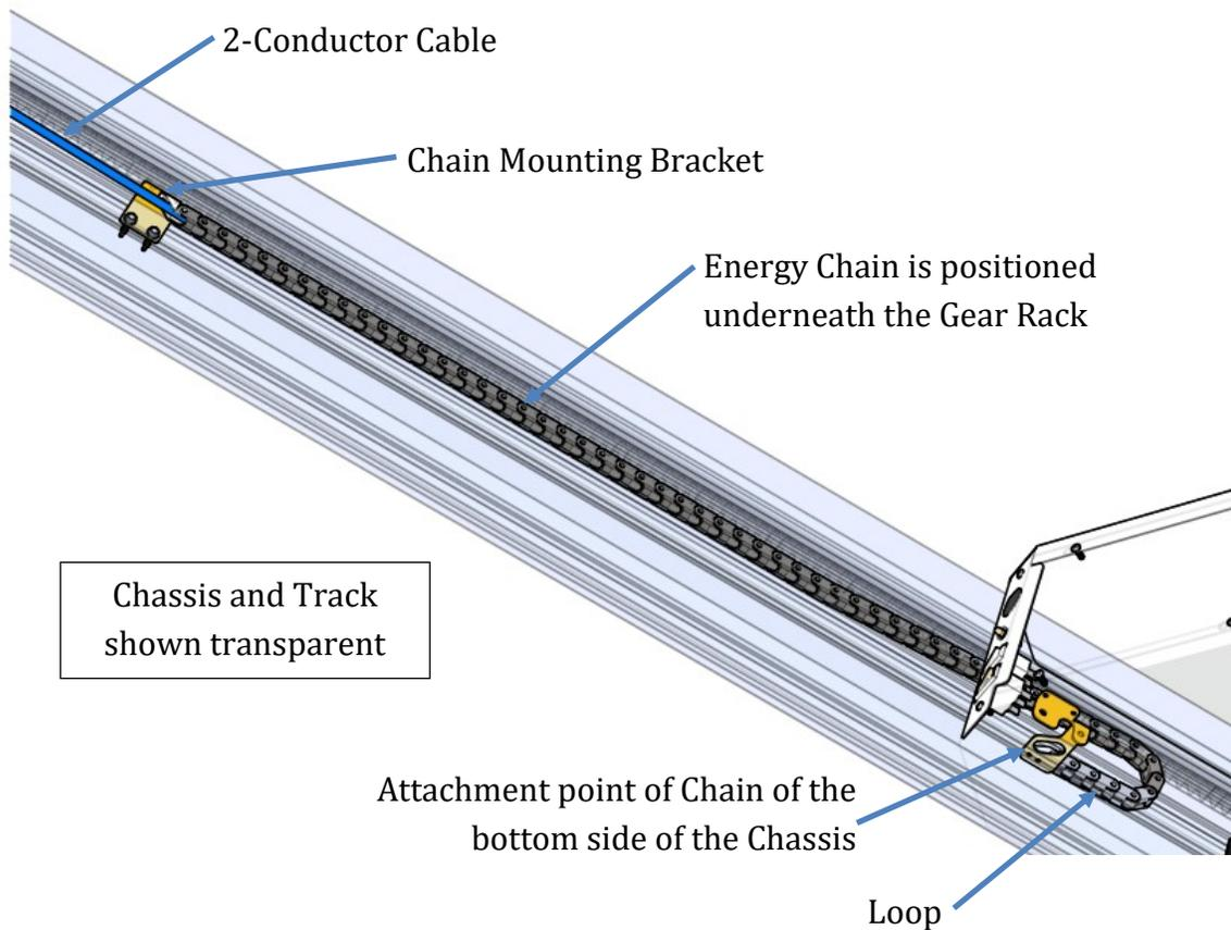
Adjust position of travel cable so there is a small loop in the Chain.
