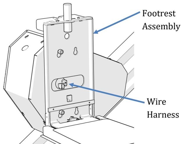
Connect the wire harness from the RF receiver to the mating connector on the backside of the chassis. Tuck the excess wiring into the opening in the chassis and mount the RF receiver to the chassis with the adhesive foam tape.
