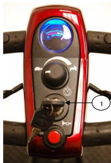
**Figure 12. Key Switch (On)**
