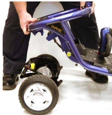
**Figure 18. Lifting the Frame**
