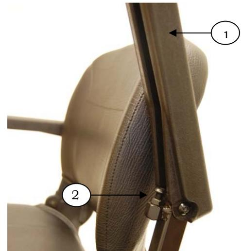
**Figure 7. Flip-up/Angle Adjustment**
