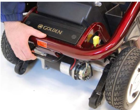
**Figure 17. Releasing the Drivetrain**
