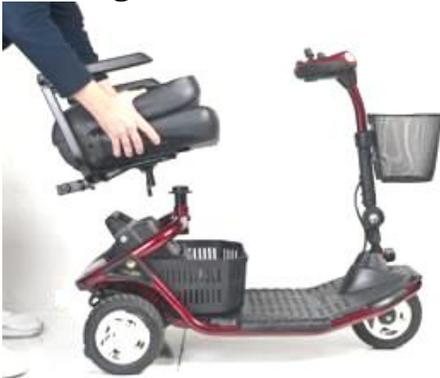
**Figure 13. Removing the Seat**
