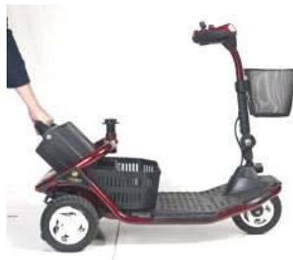
**Figure 14. Removing the Battery Pack**
