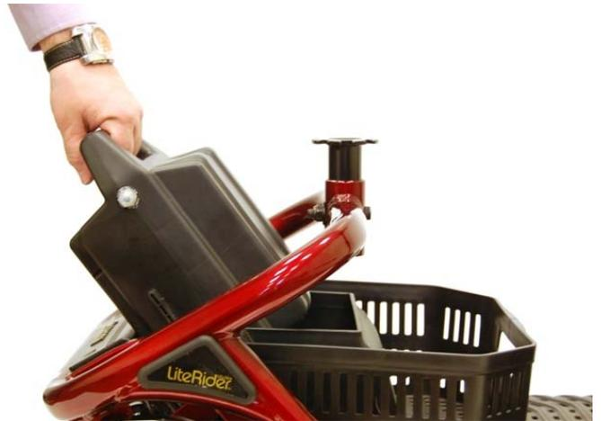
**Figure 21. Battery Pack Installation**
