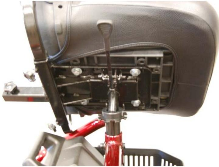
**Figure 23. Installing the Seat**
